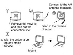
Installation hole Mount on wall, etc
