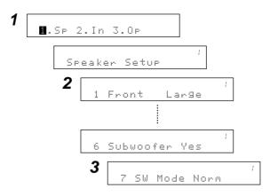
• Select "Large" or "Small" not according to the actual size of the speaker but according to the speaker's capacity for playing low frequency (bass sound below the frequency set for the Crossover Frequency) signals. If you do not know, try comparing the sound at both settings (setting the volume to a level low enough so as not to damage the speakers) to determine the proper setting.
