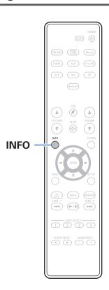
Pressing INFO on the remote control switches the display to show information such as the input source name, the volume, the sound mode name, the video input/output signals, and other information. The FRL Rate is displayed when the "4K/8K Signal Format" setting of this unit is "8K Enhanced" and the connected TV supports FRL transmission mode.
