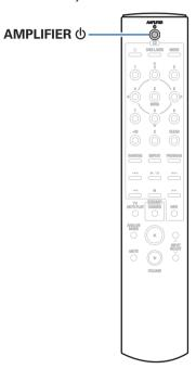
1 Press and hold AMPLIFIER (b) for 5 seconds or more to switch it on and off.
