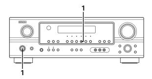
When the main unit's power operation switch turn on while pressing the set's PRESET ▲ (+) button the unit automatically begins searching for FM broadcast stations.
