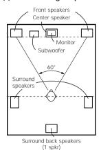
· Set the front speakers with their front surfaces as flush with the TV or monitor screen as possible. Set the center speaker between the front left and right speakers and no further from the listening position than the front speakers.
