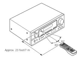
Point the remote control unit at the remote control sensor as shown on the diagram at the left.
