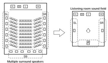
In this case it is important to achieve the same sense of expansion as in a movie theater with the surround channels. To do so, in some cases the number of surround speakers is increased (to four or eight) or speakers with bipolar or dipolar properties are used.
