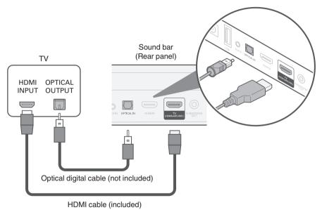
• When inserting optical digital cables, ensure that the orientation of the plugs are correct by checking the shape of the optical digital cable plugs, the OPTICAL IN connector on this unit and the optical digital connector on the unit you are connecting to. Forcible insertion in the incorrect orientation may damage the connectors and plugs.
