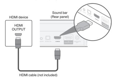
• When connecting this unit to a device that is compatible with the 4K functions, use a "High Speed HDMI cable with Ethernet" that displays the HDMI logo.
